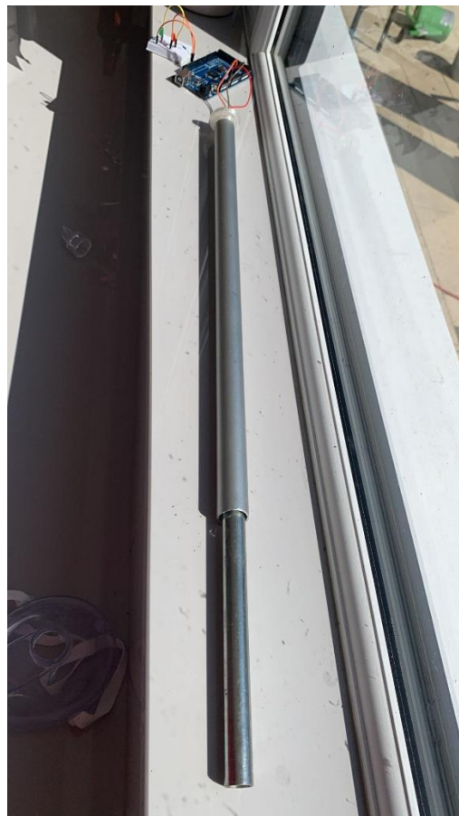
Figure 4: Sensor with Plunger
