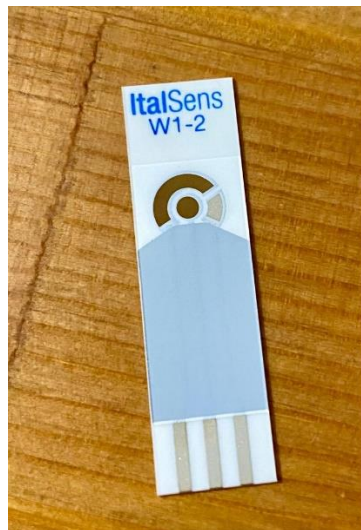
Figure 2: Electrochemical sensor used
