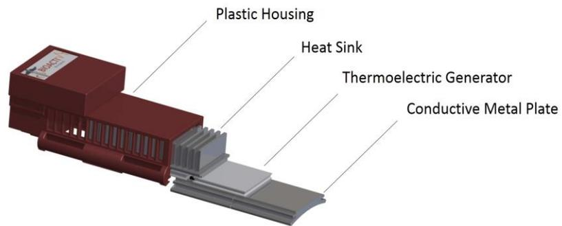
**Figure 3.** Exploded Assembly
