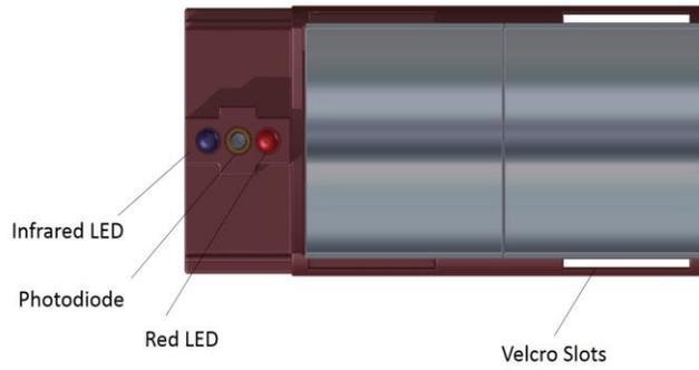
**Figure 2.** Bottom View of the Prototype
