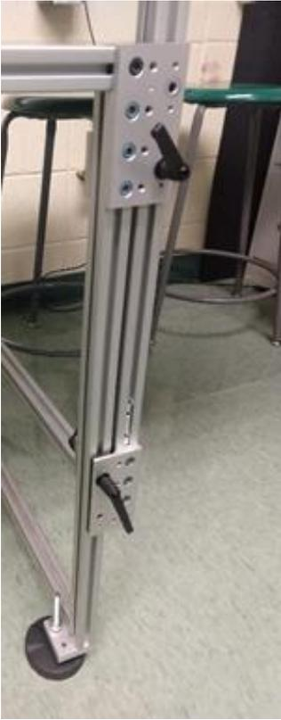
*Figure D.1 - Physical model displaying a single leg assembly*
