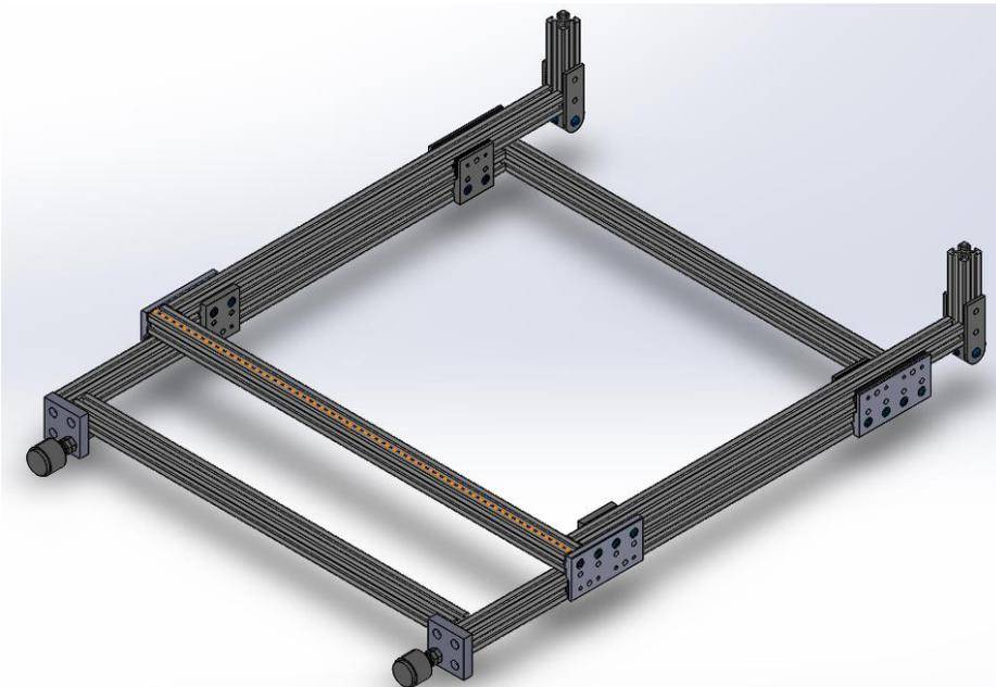
*Figure D.2 - Digital model of leg subassembly*
