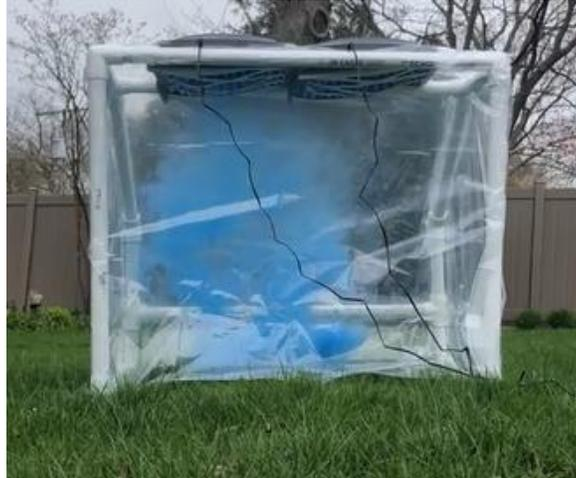
**Appendix B:** Final prototype Negative Pressure Chamber undergoing “smoke bomb” test. This test is modeled after the ASHRAE 110-2016 Standard for fume hood evaluation. As shown in the picture, smoke remains inside the enclosure and particles are not escaping the negative pressure space created by the fan and filter system.
