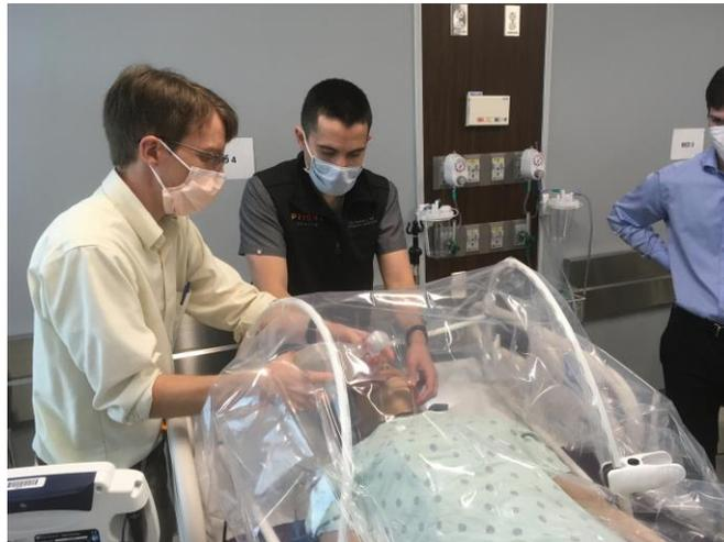
**Appendix A:** Initial prototype of the negative pressure chamber tested by PRISMA Health Emergency Medicine clinical staff. Feedback from the clinician was used to change the geometry of the opening to allow for easier access during intubation.
