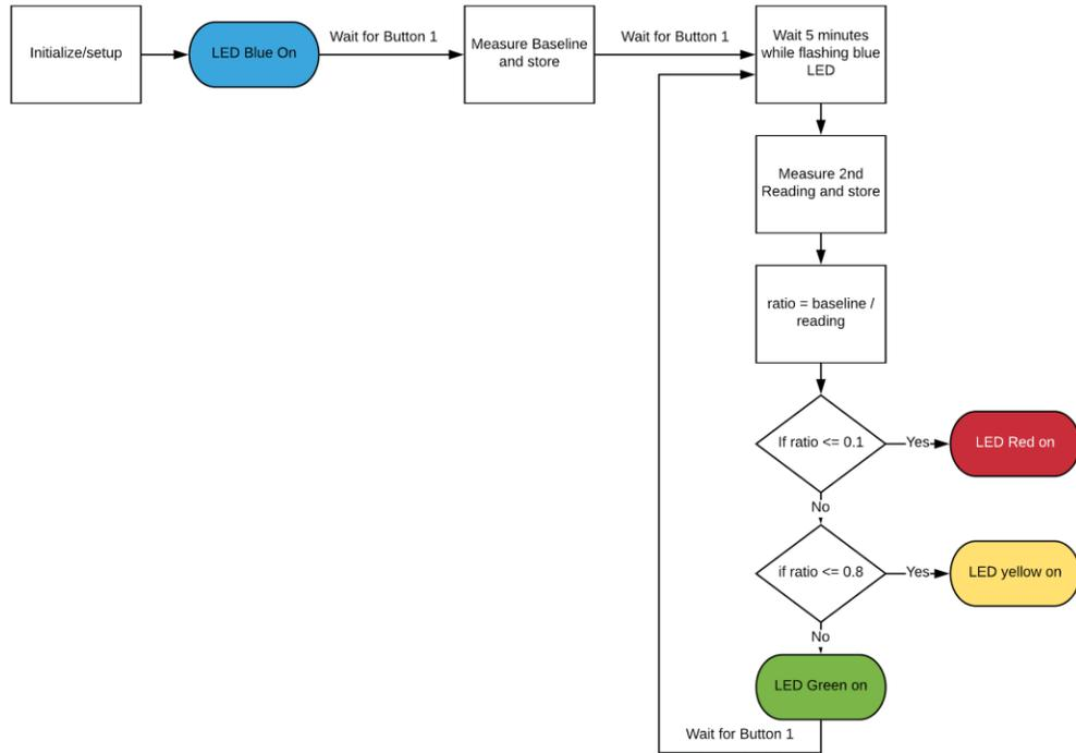
Figure 3. Code Block Diagram for Microcontroller.
