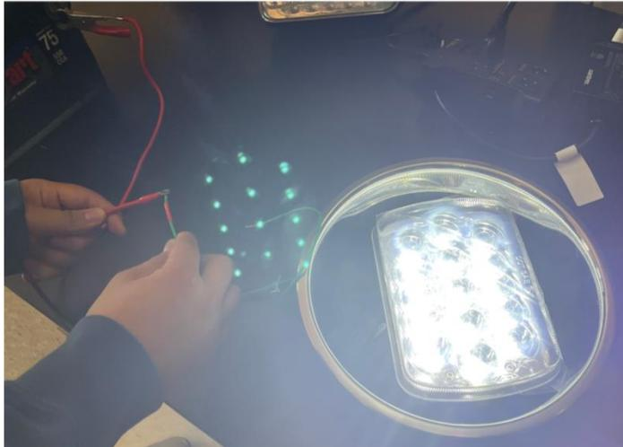
Figure 9. Illuminated headlight used for the surgical lamp
