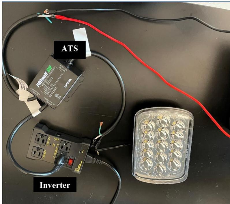
Figure 10. Built circuit containing the ATS
