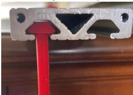
**Figure 3:** 3D-Printed Adapter in 80/20 Track
