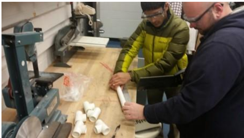
Figure 3 – Bike Pedal Generator team building a prototype frame out of PVC piping
