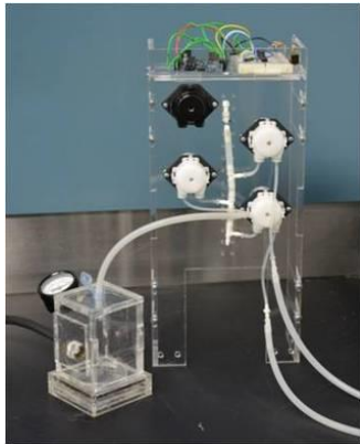
<---- Figure C: A prototype of the RNA extraction device -- one of four devices used to help diagnose HIV treatment failure.
